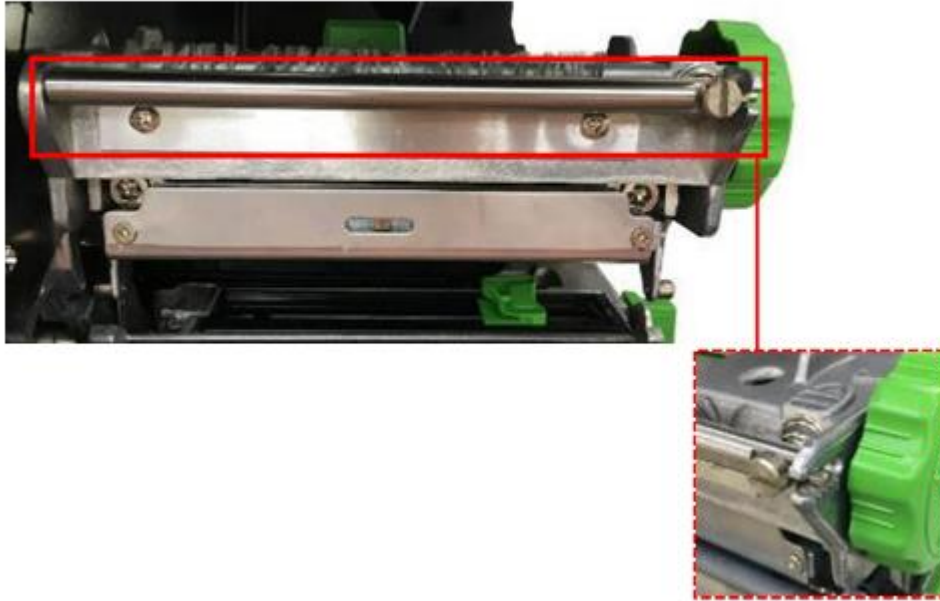
Ribbon Tension Adjustment Knob
